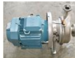
Reference: SUN-051 CENTRIFUGAL PUMP Year: 2005 Brand: APV
