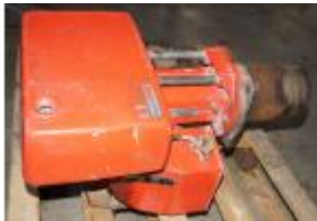
Reference: CAO-018 DIESEL BURNER FOR BOILER Year: . Brand: ROCA
