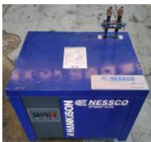
Reference: EDM-005 COMPRESSED AIR DRYER Year: 2001 Brand: HANKISON
